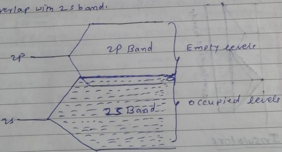
The lower energy state molecular orbitals ~~are~~ are called as valence band and Higher energy state molecular orbitals are called as conduction band.
